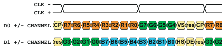
Figure 8-5. Data and Clock Input in 2-ChM (LS0 = high; LS1 = low)
