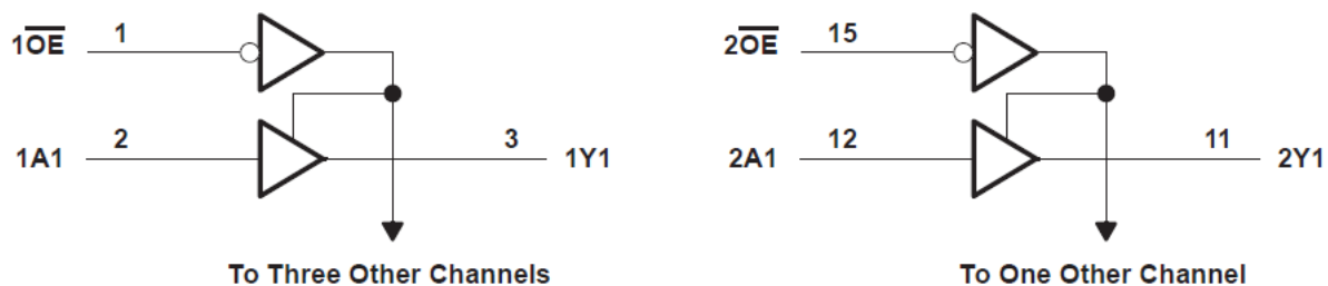
8-1. Logic Diagram (Positive Logic)
