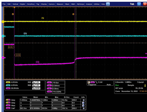
9-4. OUT In Current Fault Auto Recovery, Low Side Mode
