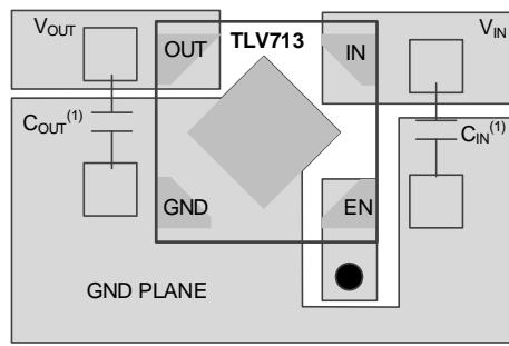
● Represents via used for application-specific connections
