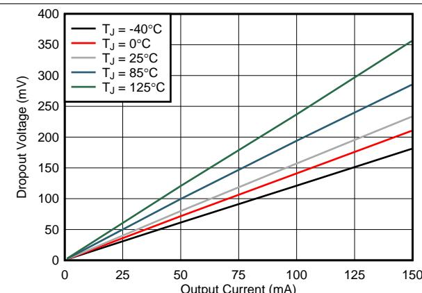
**Figure 5.** 3.3-V Dropout Voltage vs
