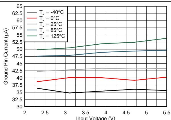
**Figure 6.** Ground Pin Current vs
