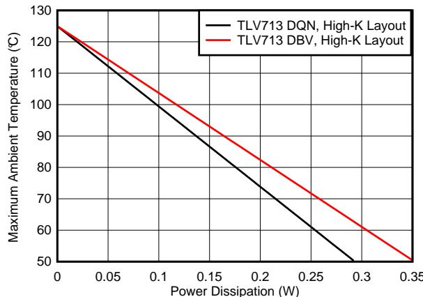
**Figure 30. Maximum Ambient Temperature vs Device Power Dissipation**
