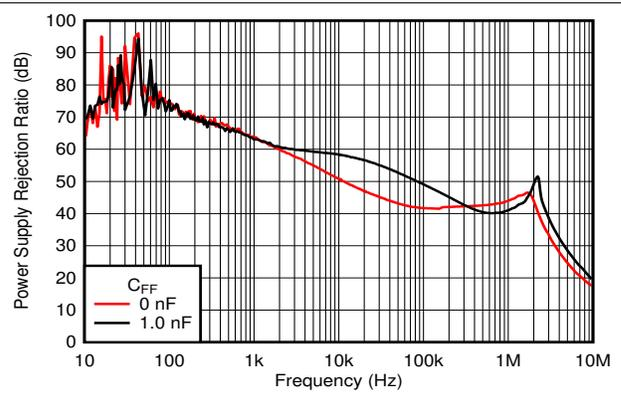
$V_{OUT} = 3.3\text{ V}$ ,  $V_{IN} = 4.8\text{ V}$ ,  $I_{OUT} = 0.33\text{ A}$
