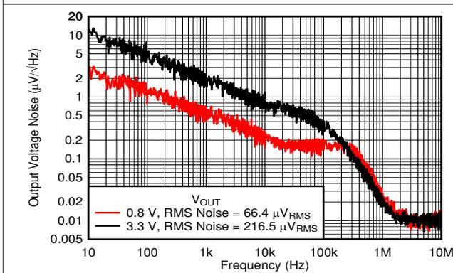
$C_{FF} = 0\text{ nF}$ ,  $I_{OUT} = 0.1\text{ A}$ , RMS noise BW = 10 Hz to 100 kHz
