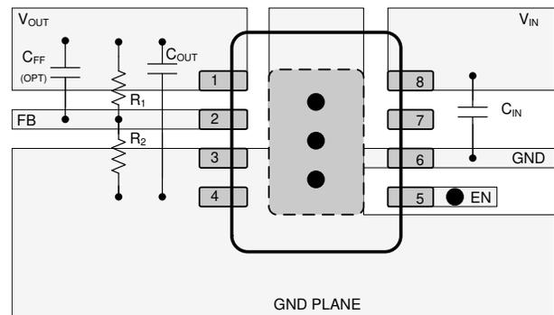
● Represents via used for application-specific connections
