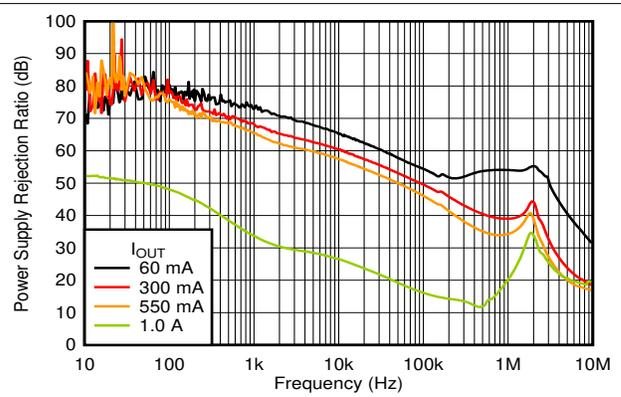
$V_{OUT} = 1.8\text{ V}$ ,  $V_{IN} = 3.3\text{ V}$ ,  $C_{FF} = 1\text{ nF}$
