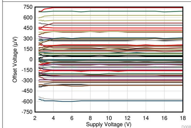
$V_{CM} = V_-$
