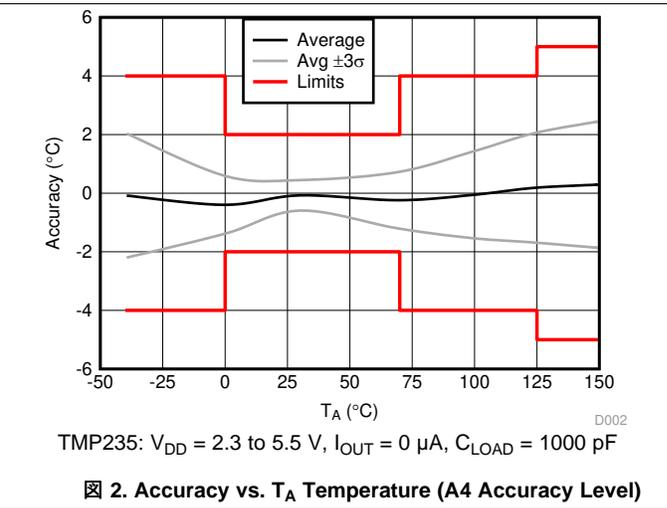
Figure 2. Accuracy vs.  $T_A$  Temperature (A4 Accuracy Level)
