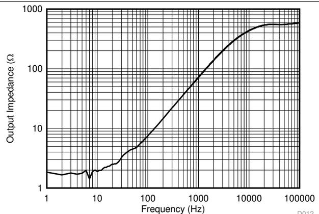
TMP235:  $T_A = 25^\circ\text{C}$ ,  $V_{DD} = 5$  V,  $I_{OUT} = 100$   $\mu\text{A}$
