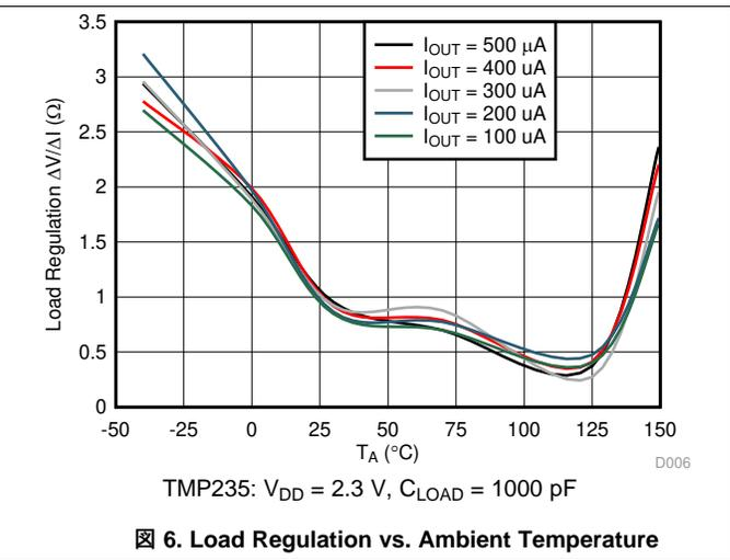
Figure 6. Load Regulation vs. Ambient Temperature
