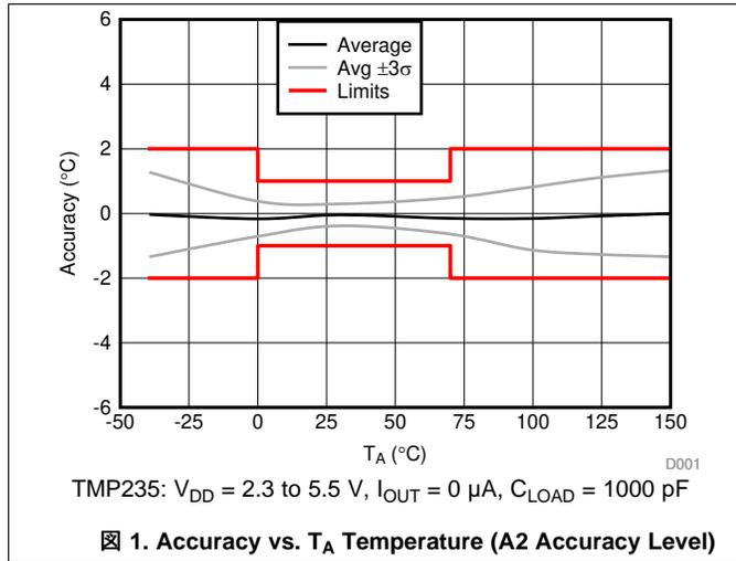
Figure 1. Accuracy vs.  $T_A$  Temperature (A2 Accuracy Level)
