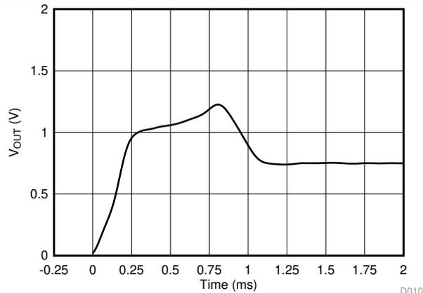
TMP235:  $T_A = 25^\circ\text{C}$ ,  $V_{DD}$  Ramp Rate =  $5$  V/ms
