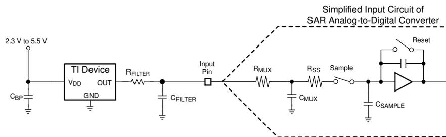
Figure 13. Suggested Connections to an ADC Input Stage
