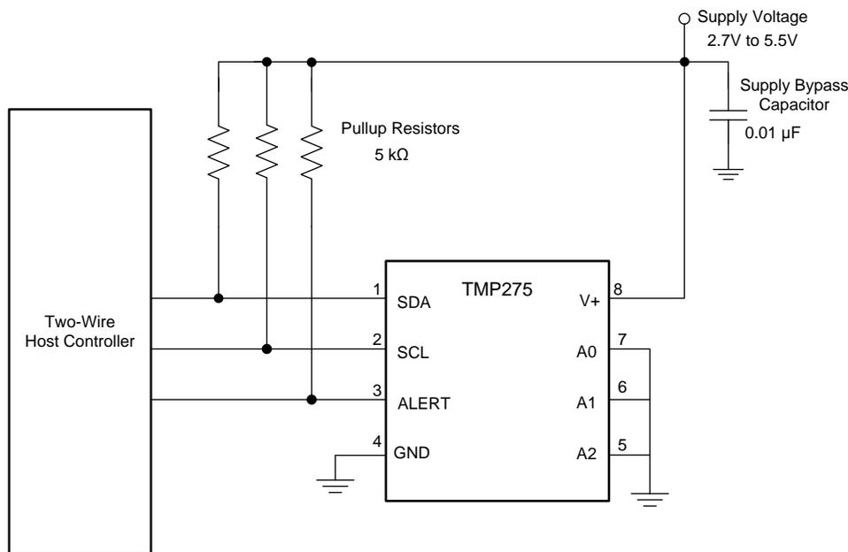
Figure 16. Typical Connections of the TMP275 Schematic
