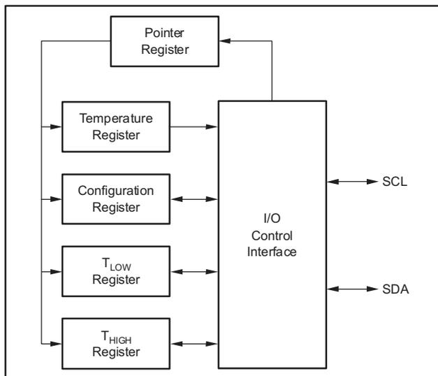
Figure 11. Internal Register Structure of the TMP275
