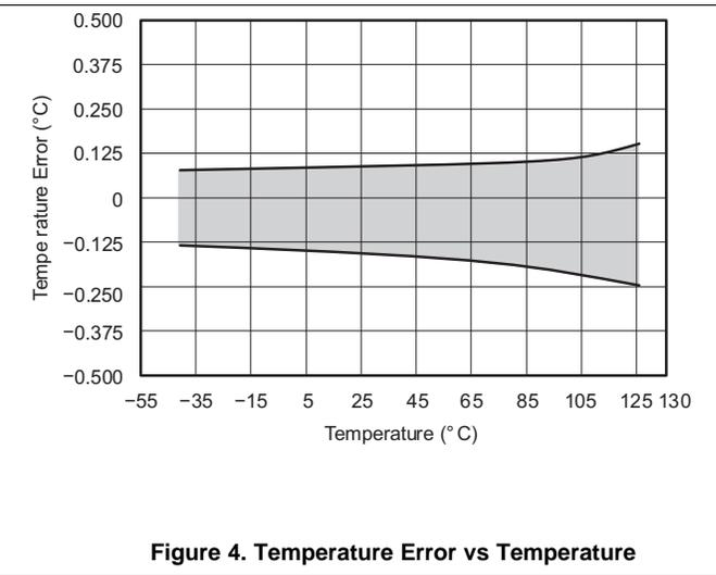
Figure 4. Temperature Error vs Temperature
