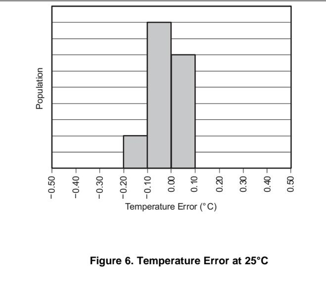
Figure 6. Temperature Error at 25°C
