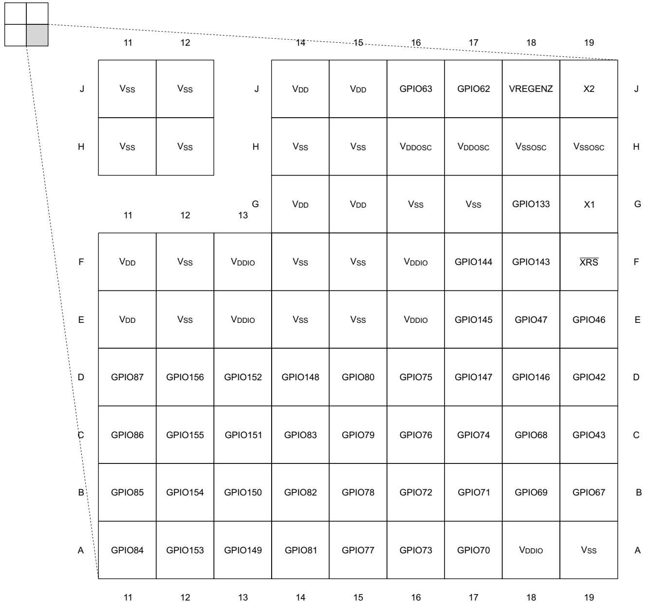
Figure 3-3. 337-Ball ZWT New Fine Pitch Ball Grid Array (Bottom View) – [Quadrant C]
