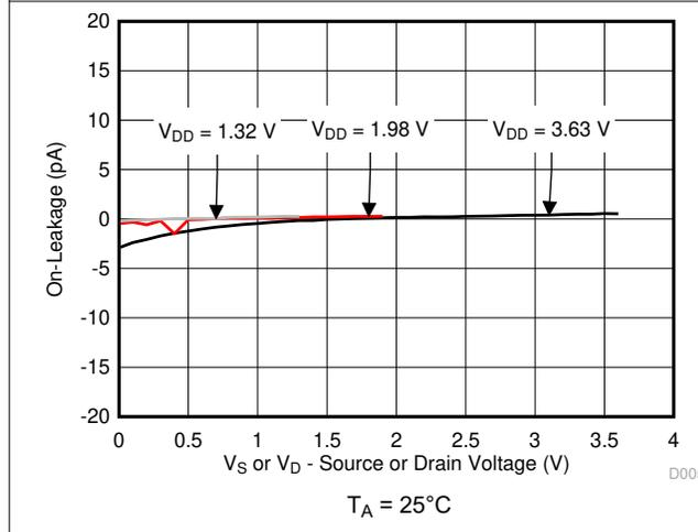
Figure 6-5. On-Leakage vs Source or Drain Voltage
