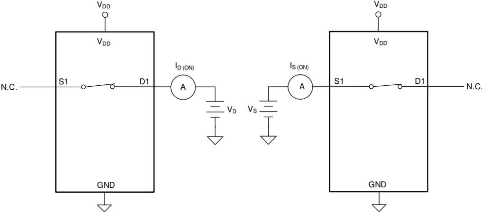
7-3 shows the circuit used for measuring the on-leakage current, denoted by  $I_{S(ON)}$  or  $I_{D(ON)}$ .
