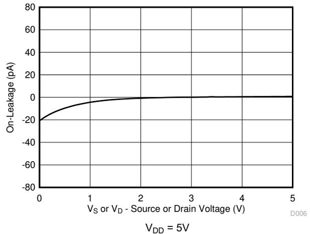
**Figure 9-3. On-Leakage vs Source or Drain Voltage**
