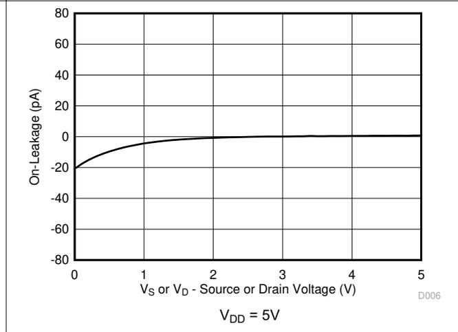
Figure 6-6. On-Leakage vs Source or Drain Voltage
