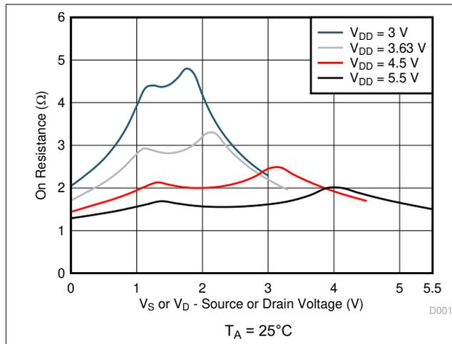
Figure 6-1. On-Resistance vs Source or Drain Voltage
