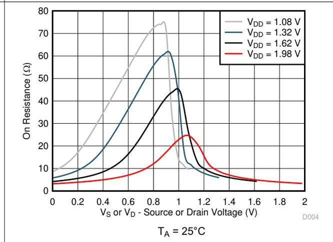
Figure 6-4. On-Resistance vs Source or Drain Voltage
