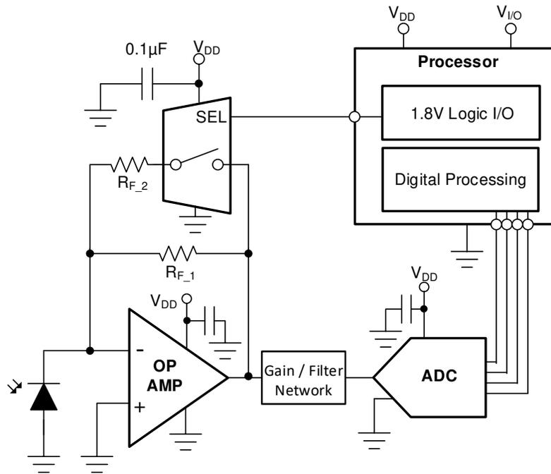
図 9-4. Configurable Gain Setting of a TIA Circuit
