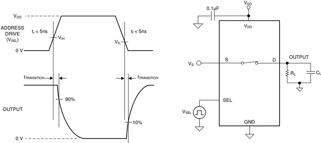
7-4 shows the setup used to measure transition time, denoted by the symbol  $t_{TRANSITION}$ .
