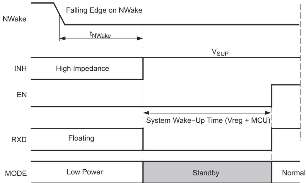
**8-3. Wake-Up Via NWake Timing Diagram**
