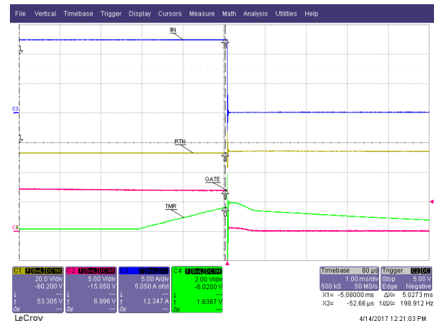
Figure 28. Output Hot Short (VinB = 60 V)
