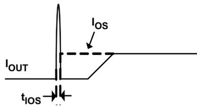
FIG 21. Response Time to Short-Circuit Waveform
