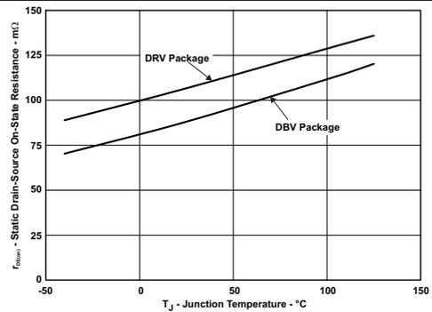
16. MOSFET  $r_{DS(on)}$  Vs. Junction Temperature
