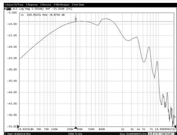
8-32. Off-State Data-Switch Isolation vs Frequency (TPS25832-Q1)
