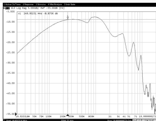
8-30. Off-State Data-Switch Isolation vs Frequency (TPS25830A-Q1)
