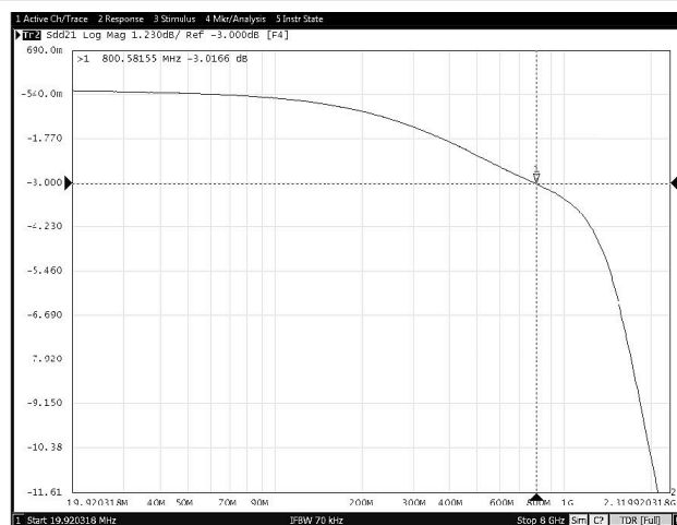
8-29. Data Transmission Characteristics vs Frequency (TPS25830A-Q1)
