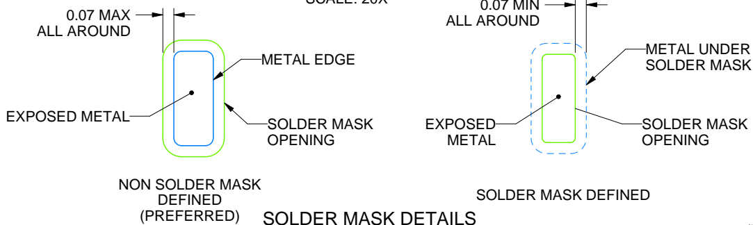
LAND PATTERN EXAMPLE EXPOSED METAL SHOWN SCALE: 20X
