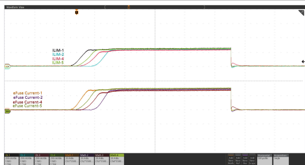
Figure 9-8. Power Up into Short (Current distribution among five devices in parallel): V_{IN} = 12 V, EN/UVLO Stepped Up From 0 V to 3 V, R_{REF} = 40.2 k \Omega , R_{ILIM} on Each Device = 300 \Omega , and OUT Shorted to GND
