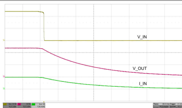
Figure 10-9. Power Fail With 24-Ω Load—Supports 1-A Load for 10-ms Power Fail
