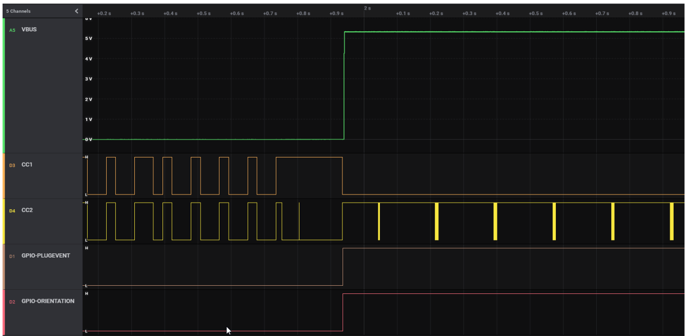
図 8-21. USB SuperSpeed Mux Control - Flipped Orientation
