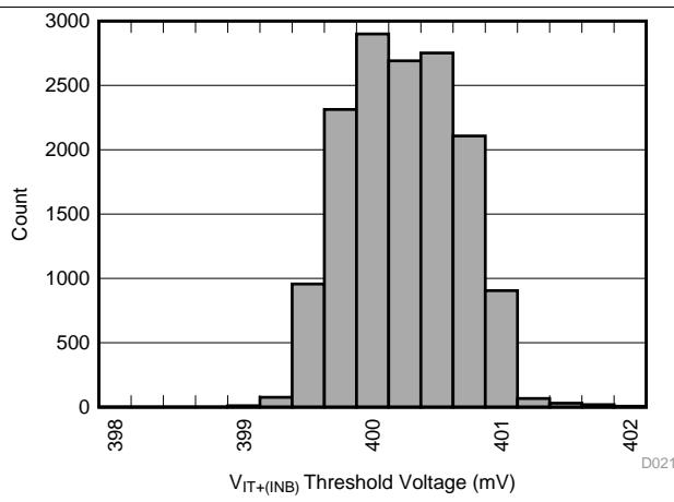
Figure 10. INB Positive Input Threshold Voltage ( $V_{IT+(INB)}$ ) Distribution
