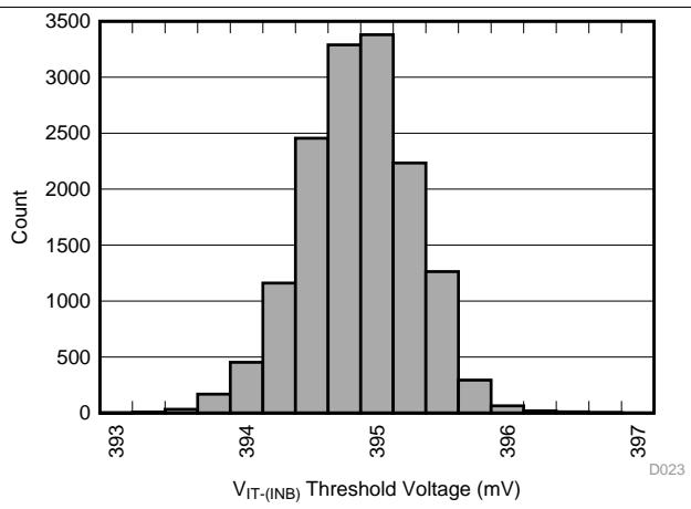
Figure 11. INB Negative Input Threshold Voltage ( $V_{IT-(INB)}$ ) Distribution
