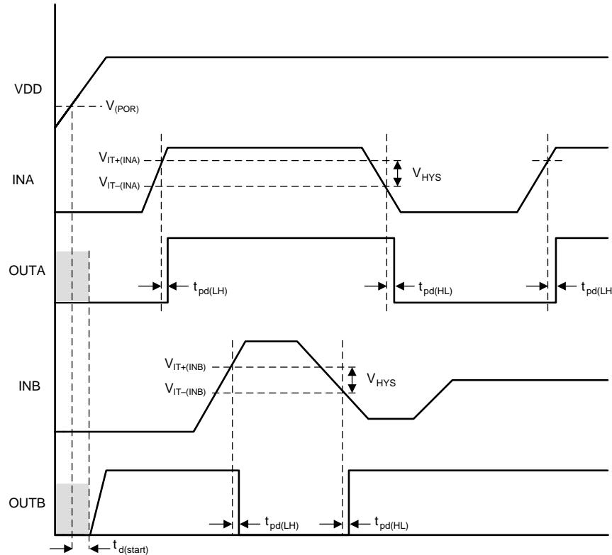
Figure 1. Timing Diagram
