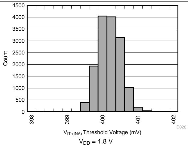
Figure 9. INA Negative Input Threshold Voltage ( $V_{IT-(INA)}$ ) Distribution
