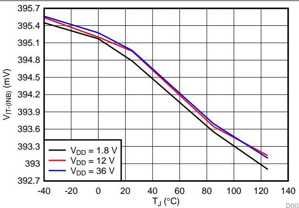
**Figure 7. INB Negative Input Threshold Voltage ( $V_{IT-}(INB)$ ) vs Temperature**
