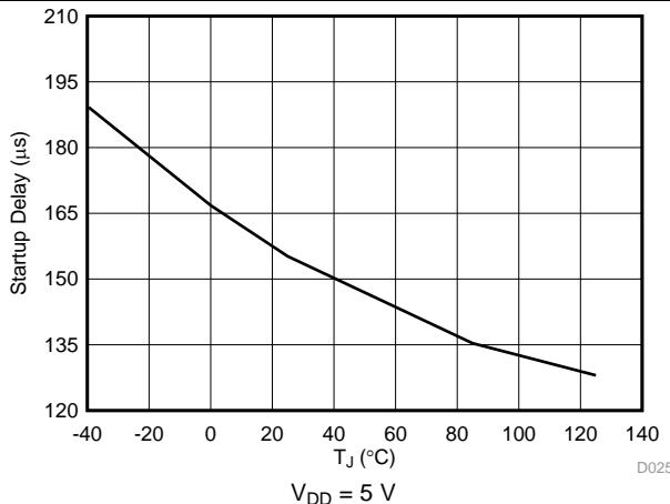
**Figure 16. Start-Up Delay vs Temperature**
