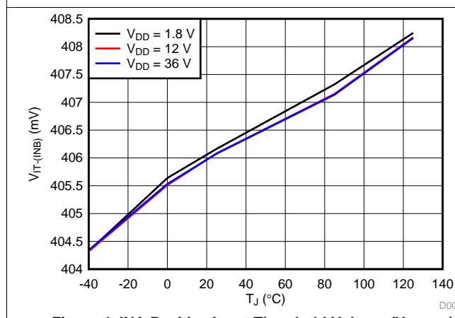
**Figure 4. INA Positive Input Threshold Voltage ( $V_{IT+}(INA)$ ) vs Temperature**
