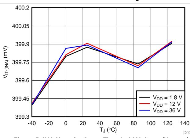
**Figure 5. INA Negative Input Threshold Voltage ( $V_{IT-}(INA)$ ) vs Temperature**
