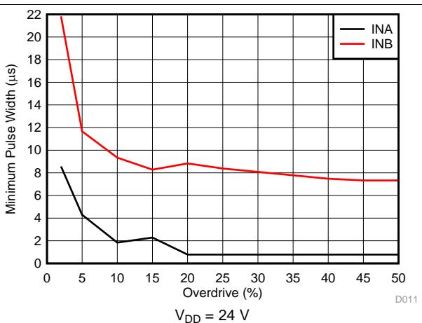
**Figure 3. Minimum Pulse Duration vs Threshold Overdrive Voltage<sup>(1)</sup> (1)**
