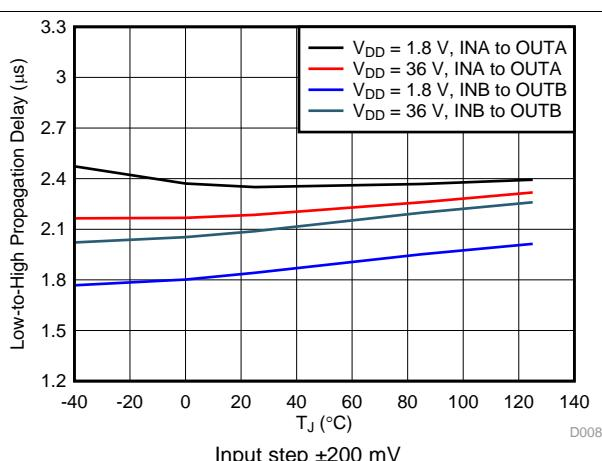
Figure 13. Propagation Delay vs Temperature (Low-to-High Transition at the Inputs)
