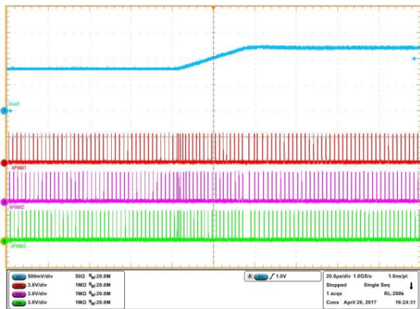
V_{VIN} = 12\text{ V} I_{VOUT\_A} = 30\text{ A} V_{OUT\_A} VID step from 0.8 V to 1.2 V
