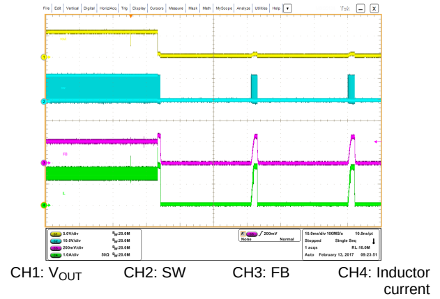
図 35. LED Short Protection (100% PWM Duty Cycle) of TPS54201
