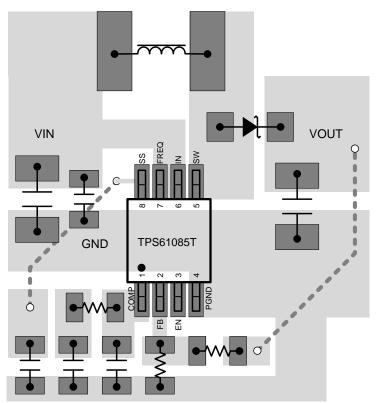
Figure 22. TPS61085T Layout Example
