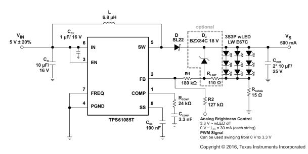
Figure 21. Simple Application (3.3-V Input –  $f_{sw}$  = 650 kHz) for wLED Supply (3S3P) With Adjustable Brightness Control Using an Analog Signal on the Feedback Pin (With Optional Clamping Zener Diode)
