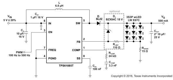
Figure 20. Simple Application (3.3-V Input – f<sub>sw</sub> = 650 kHz) for wLED Supply (3S3P) With Adjustable Brightness Control using a PWM Signal on the Enable Pin (With Optional Clamping Zener Diode)
