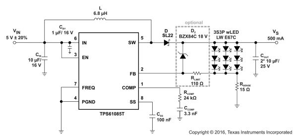
Figure 19. Simple Application (3.3-V Input – f<sub>sw</sub> = 650 kHz) for wLED Supply (3S3P) (With Optional Clamping Zener Diode)
