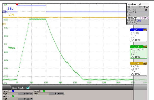
FIG 8-40. Short Circuit Behavior
