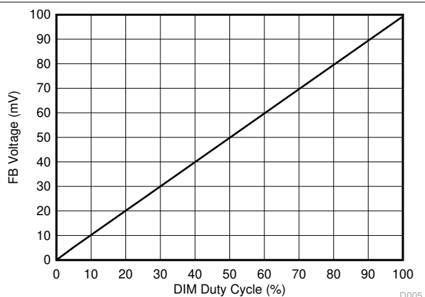
FIG 6-5. DIM Duty Cycle vs FB Voltage in Analog Dimming (for TPS92200D2)
