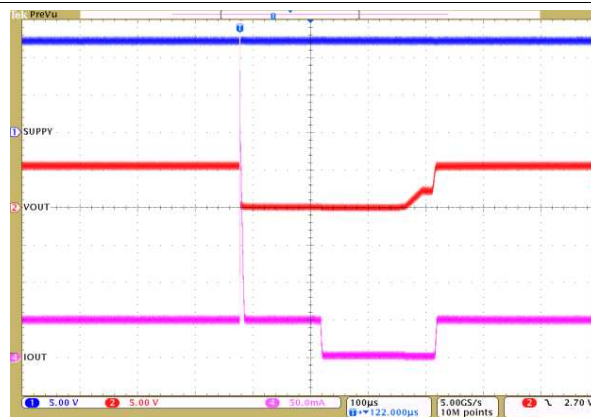
図 11. LED Short-Circuit Protection and Recovery
