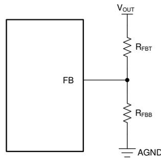
**図 7-8. Setting Output Voltage for Adjustable Output Variant**
