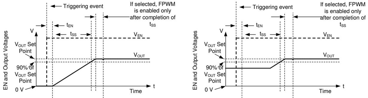
**Figure 7-9. Soft Start With and Without Pre-biased Voltage**
