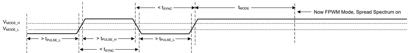
图 7-5. Transition from SYNC Mode to FPWM Mode
