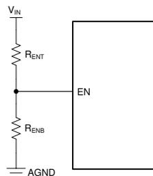
**図 7-2.  $V_{IN}$  Undervoltage Lockout Using the EN/UVLO Pin**
