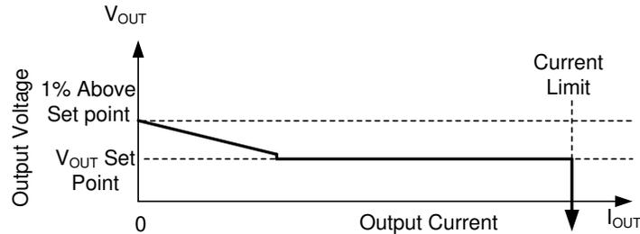
In auto mode, after output current drops below approximately 1/10th the rated current of the part, output resistance increases so that output voltage is 1% high while the buck is completely unloaded.
