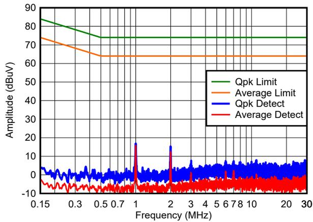
$V_{IN} = 24\text{ V}$       $V_{OUT} = 5\text{ V}$       $F_{sw} = 1\text{ MHz}$
