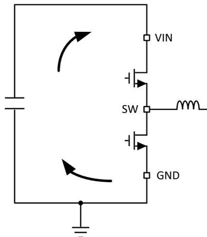
图 8-15. Current Loops with Fast Edges
