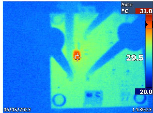
$V_{IN} = 24\text{ V}$       $V_{OUT} = 5\text{ V}$      150 mA, 1 MHz
