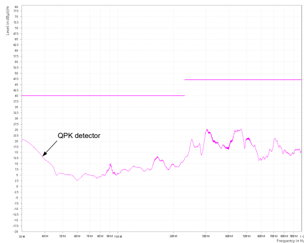
Figure 9-10. CISPR 32 Class B Radiated Emissions: Horizontal Polarization
