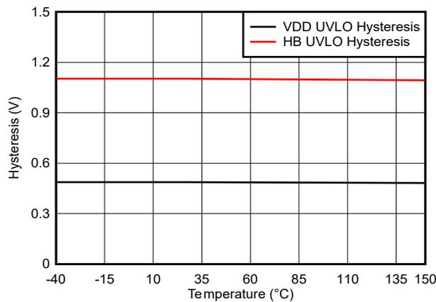
Figure 5-10. Undervoltage Lockout Threshold Hysteresis vs Temperature
