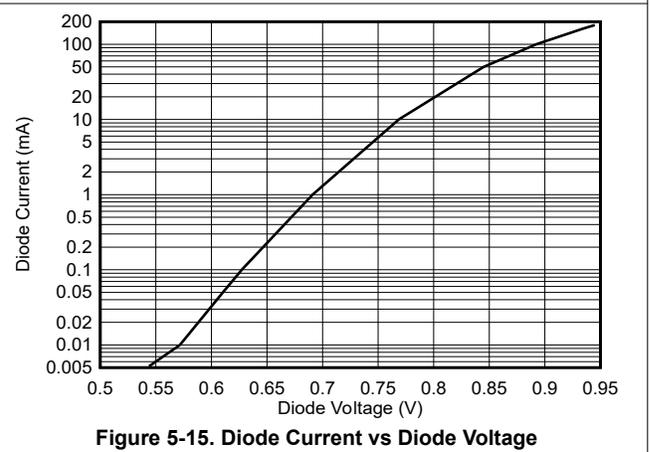
Figure 5-15. Diode Current vs Diode Voltage
