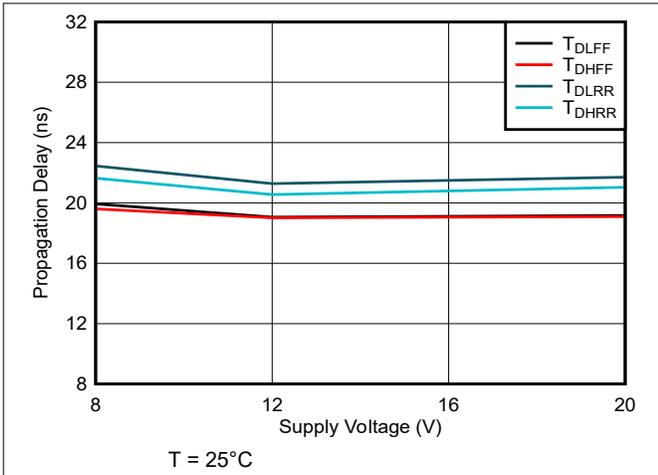
Figure 5-12. Propagation Delays vs Supply Voltage ( $V_{DD} = V_{HB}$ )
