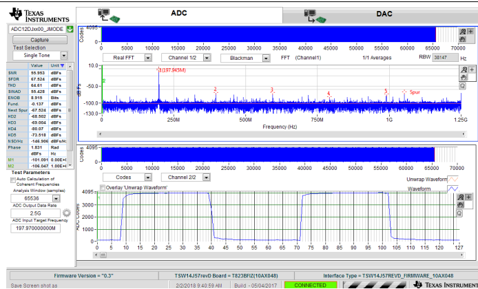
Figure 191. 200-MHz, Sine-Wave (Channel A) Frequency Domain (FFT) and 40-MHz, Square-Wave (Channel B) Time Domain for 5-GSPS, Single-Channel Oscilloscope
