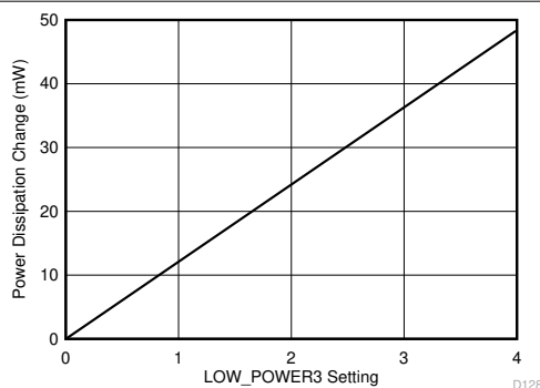
図 6-13. Power Dissipation Change vs LOW_POWER3 register setting
