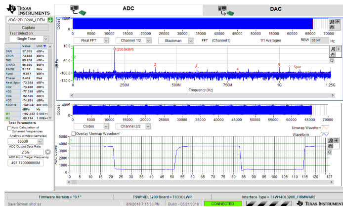
8-11. 200-MHz, Sine-Wave (Channel A) Frequency Domain (FFT) and 40-MHz, Square-Wave (Channel B) Time Domain for 5-GSPS, Single-Channel Oscilloscope
