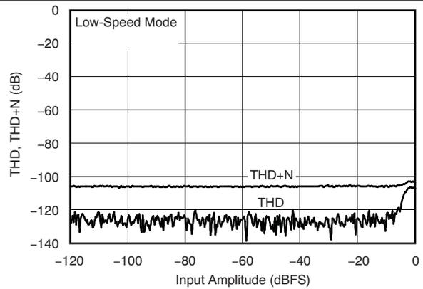
Figure 26. Total Harmonic Distortion vs Input Amplitude
