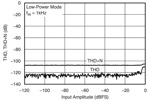
Figure 24. Total Harmonic Distortion vs Input Amplitude
