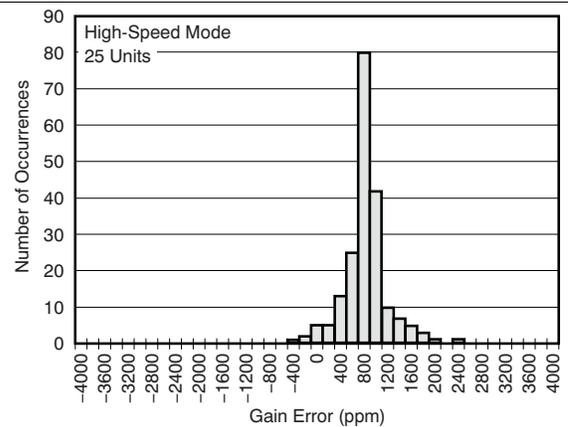
Figure 32. Gain Error Histogram
