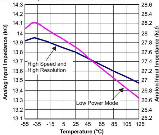
Figure 39. Analog Input Differential Impedance vs Temperature
