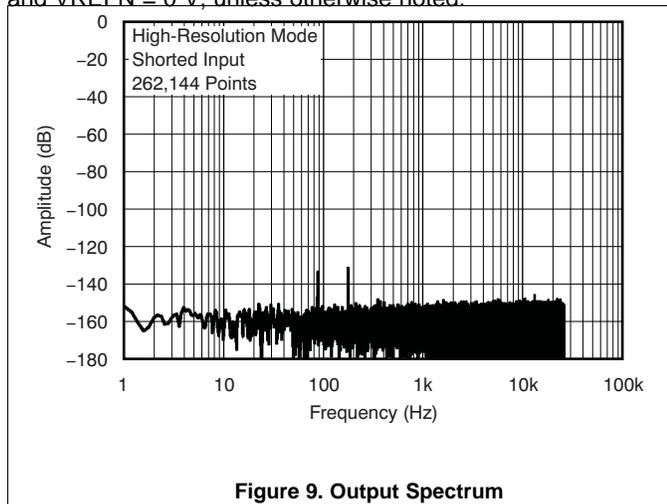
Figure 9. Output Spectrum
