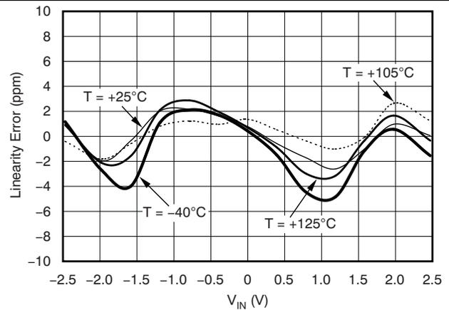
Figure 42. Linearity Error vs Input Level
