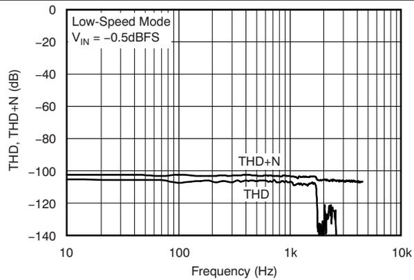
Figure 25. Total Harmonic Distortion vs Frequency
