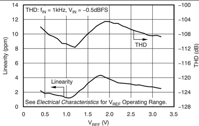
Figure 43. Linearity and Total Harmonic Distortion vs Reference Voltage
