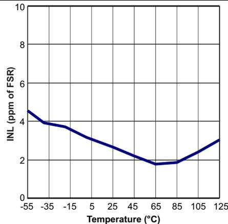
Figure 41. Integral Nonlinearity vs Temperature
