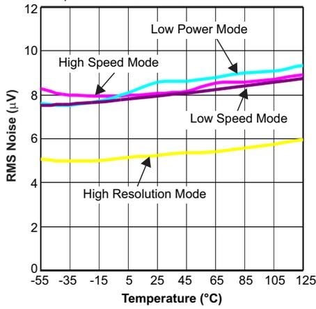
Figure 45. Noise vs Temperature
