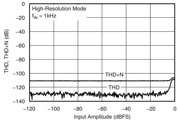
Figure 22. Total Harmonic Distortion vs Input Amplitude
