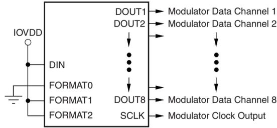
**Figure 80. Modulator Output**
