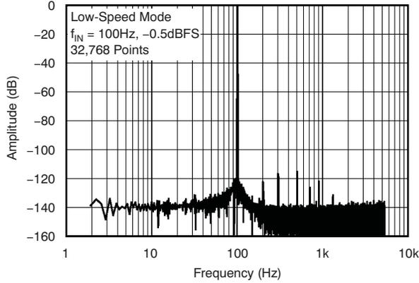
Figure 15. Output Spectrum
