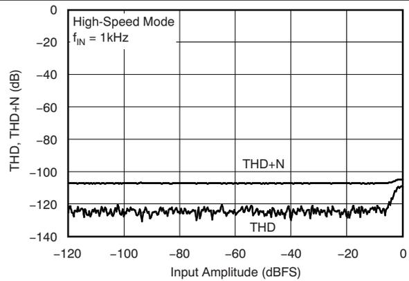
Figure 20. Total Harmonic Distortion vs Input Amplitude
