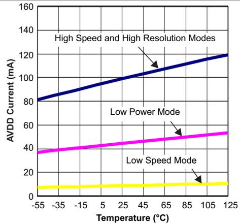
Figure 50. AVDD Current vs Temperature
