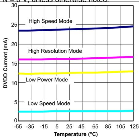
Figure 51. DVDD Current vs Temperature
