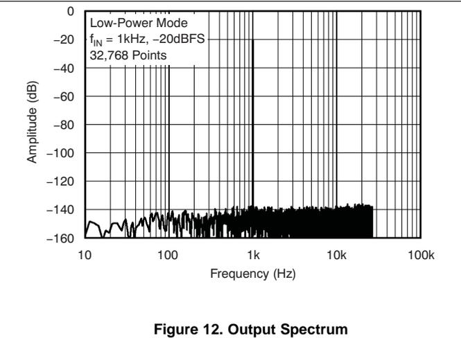
Figure 12. Output Spectrum
