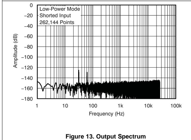
Figure 13. Output Spectrum
