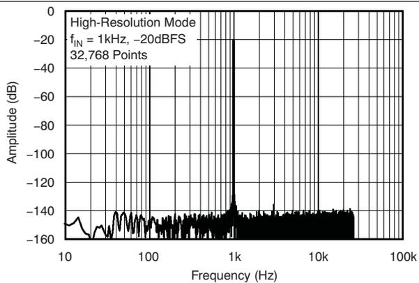
Figure 8. Output Spectrum
