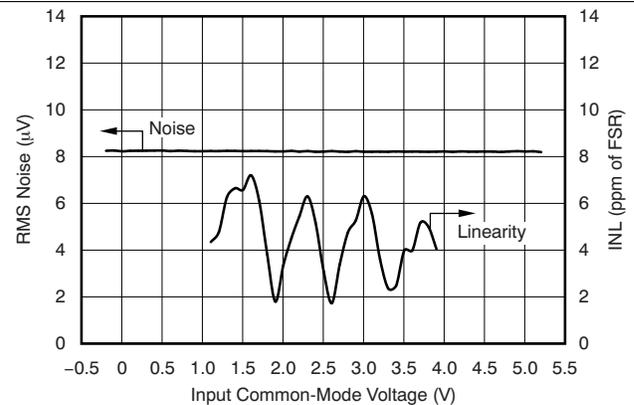
Figure 44. Noise and Linearity vs Input Common-Mode Voltage
