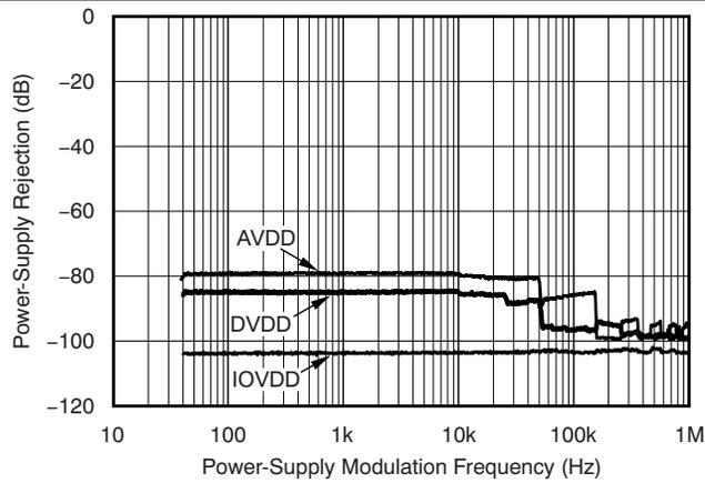
Figure 49. Power-Supply Rejection vs Power-Supply Frequency
