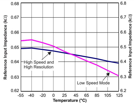
Figure 38. Reference Input Differential Impedance vs Temperature
