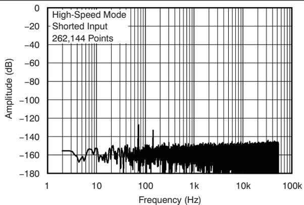
Figure 5. Output Spectrum
