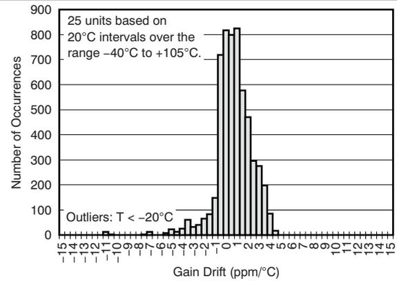
Figure 28. Gain Drift Histogram
