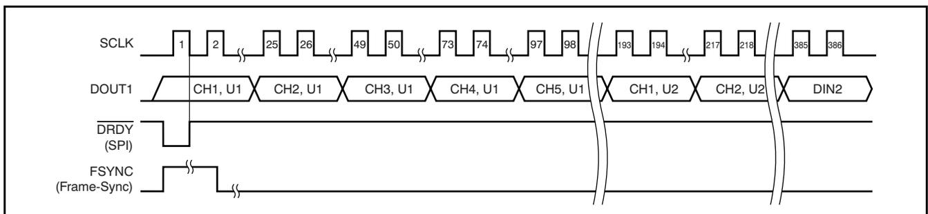
**Figure 78. Daisy-Chain Data Format of Figure 77**
