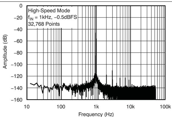
Figure 3. Output Spectrum
