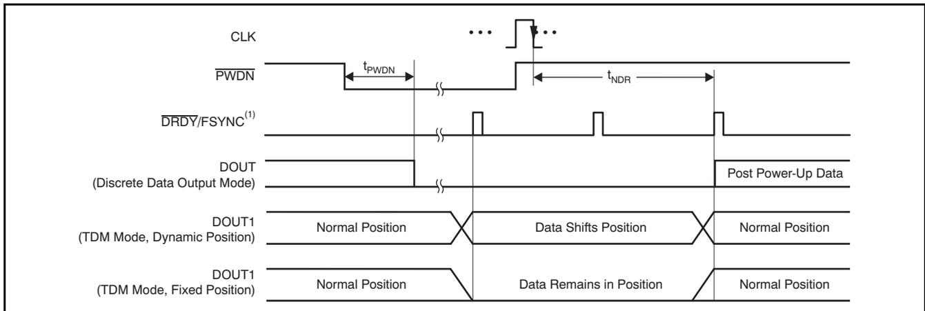
Figure 71. Power-Down Timing
