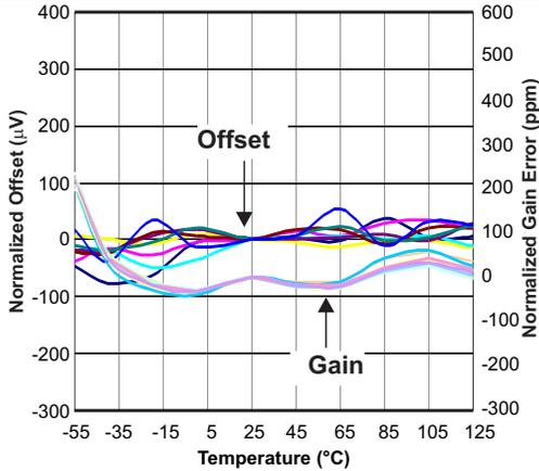
Figure 35. Offset and Gain vs Temperature
