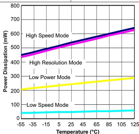
Figure 53. Power Dissipation vs Temperature
