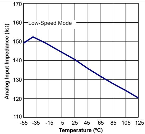
Figure 40. Analog Input Differential Impedance vs Temperature
