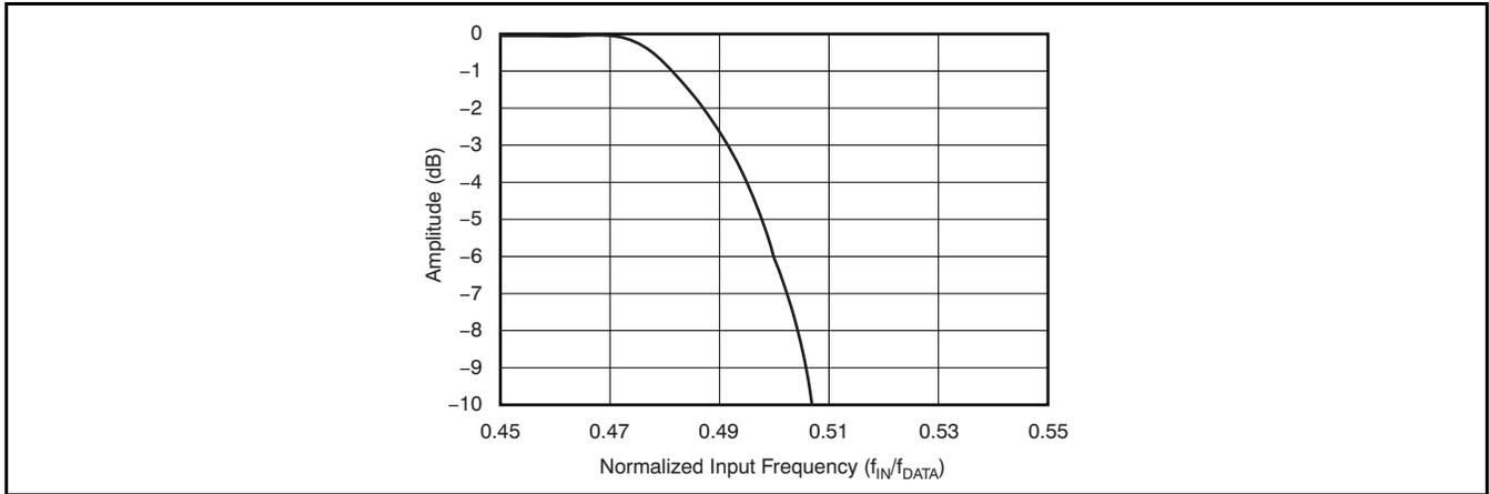
Figure 60. Transition Band Response For High-Resolution Mode
