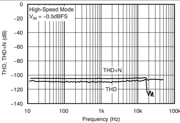
Figure 19. Total Harmonic Distortion vs Frequency
