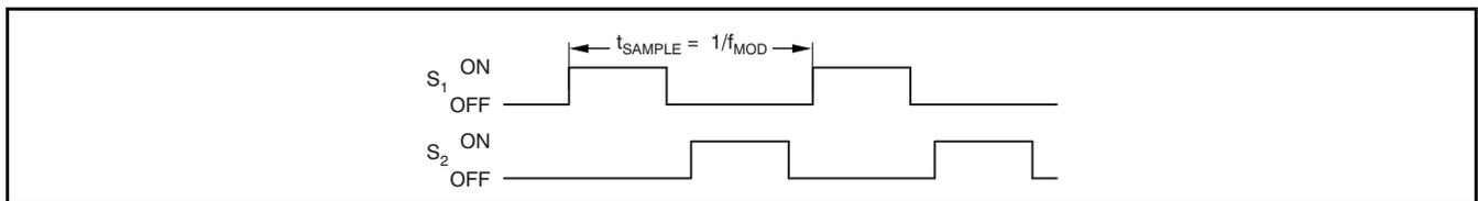
Figure 64.  $S_1$  and  $S_2$  Switch Timing for Figure 63
