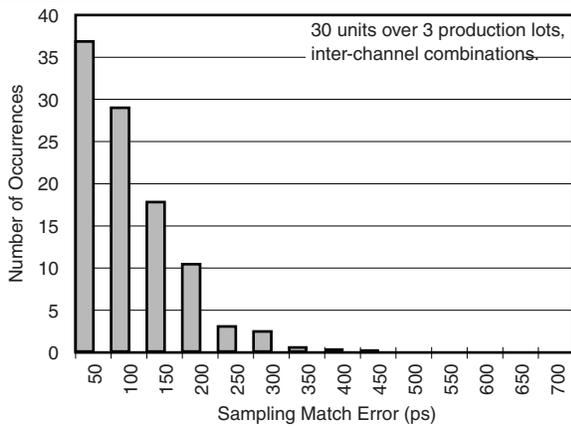
Figure 37. Sampling Match Error Histogram
