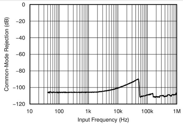
Figure 48. Common-Mode Rejection vs Input Frequency
