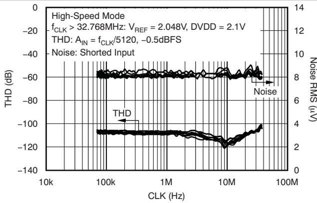
Figure 47. Total Harmonic Distortion and Noise vs CLK
