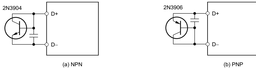
☒ 7-6. Remote Temperature Sensor Using Transistor
