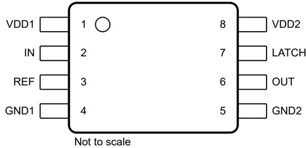
**Figure 4-1. DWV Package, 8-Pin SOIC (Top View)**
