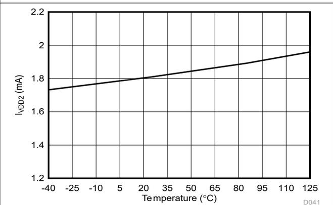
Figure 5-33. Low-Side Supply Current vs Temperature
