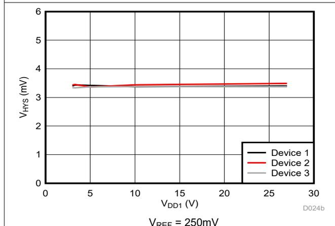
Figure 5-16. Trip Threshold Hysteresis vs Supply Voltage
