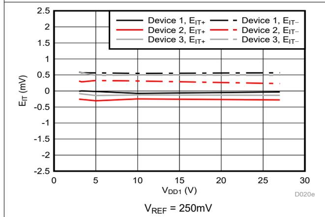
Figure 5-14. Trip Threshold Error vs Supply Voltage
