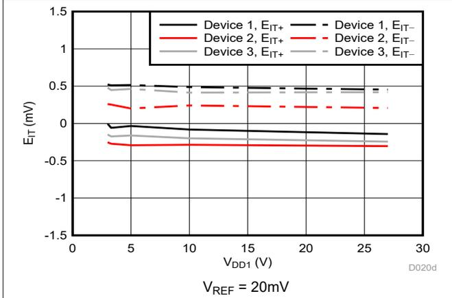
Figure 5-8. Trip Threshold Error vs Supply Voltage
