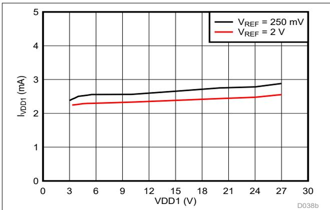
Figure 5-30. High-Side Supply Current vs Supply Voltage
