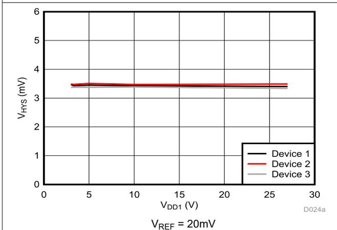
Figure 5-10. Trip Threshold Hysteresis vs Supply Voltage
