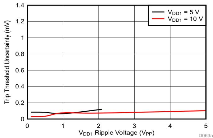
Figure 7-3. Trip Threshold Sensitivity to VDD1 Ripple Voltage (f<sub>RIPLLE</sub> = 10kHz)
