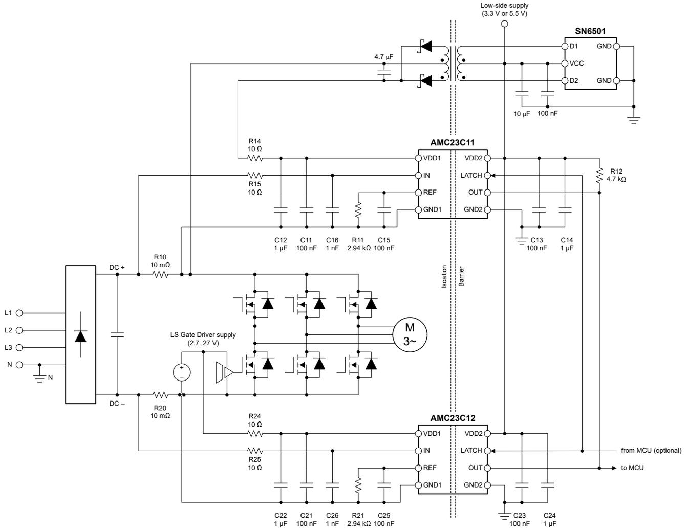
Figure 7-1. Using the AMC23C11 for DC+ Overcurrent Detection
