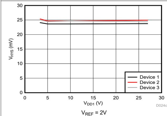
Figure 5-22. Trip Threshold Hysteresis vs Supply Voltage
