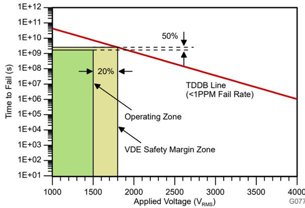
TA up to 150°C, stress-voltage frequency = 60Hz, isolation working voltage = 1000VRMS, operating lifetime > 400 years
