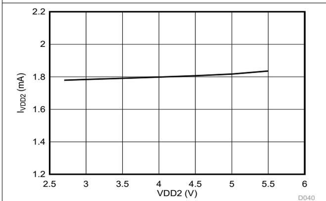
Figure 5-32. Low-Side Supply Current vs Supply Voltage
