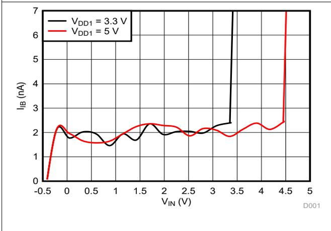
Figure 5-26. Input Bias Current vs Input Voltage
