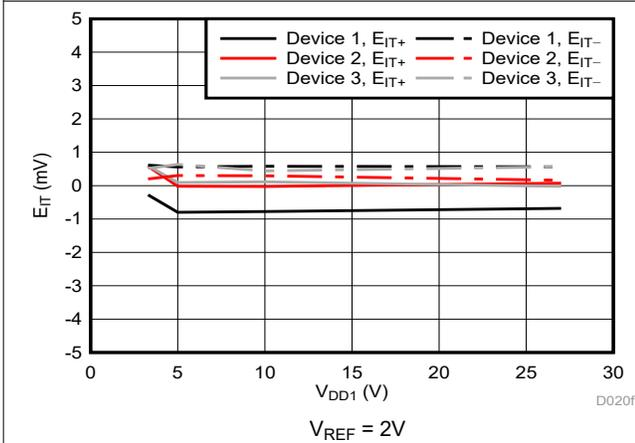
Figure 5-20. Trip Threshold Error vs Supply Voltage
