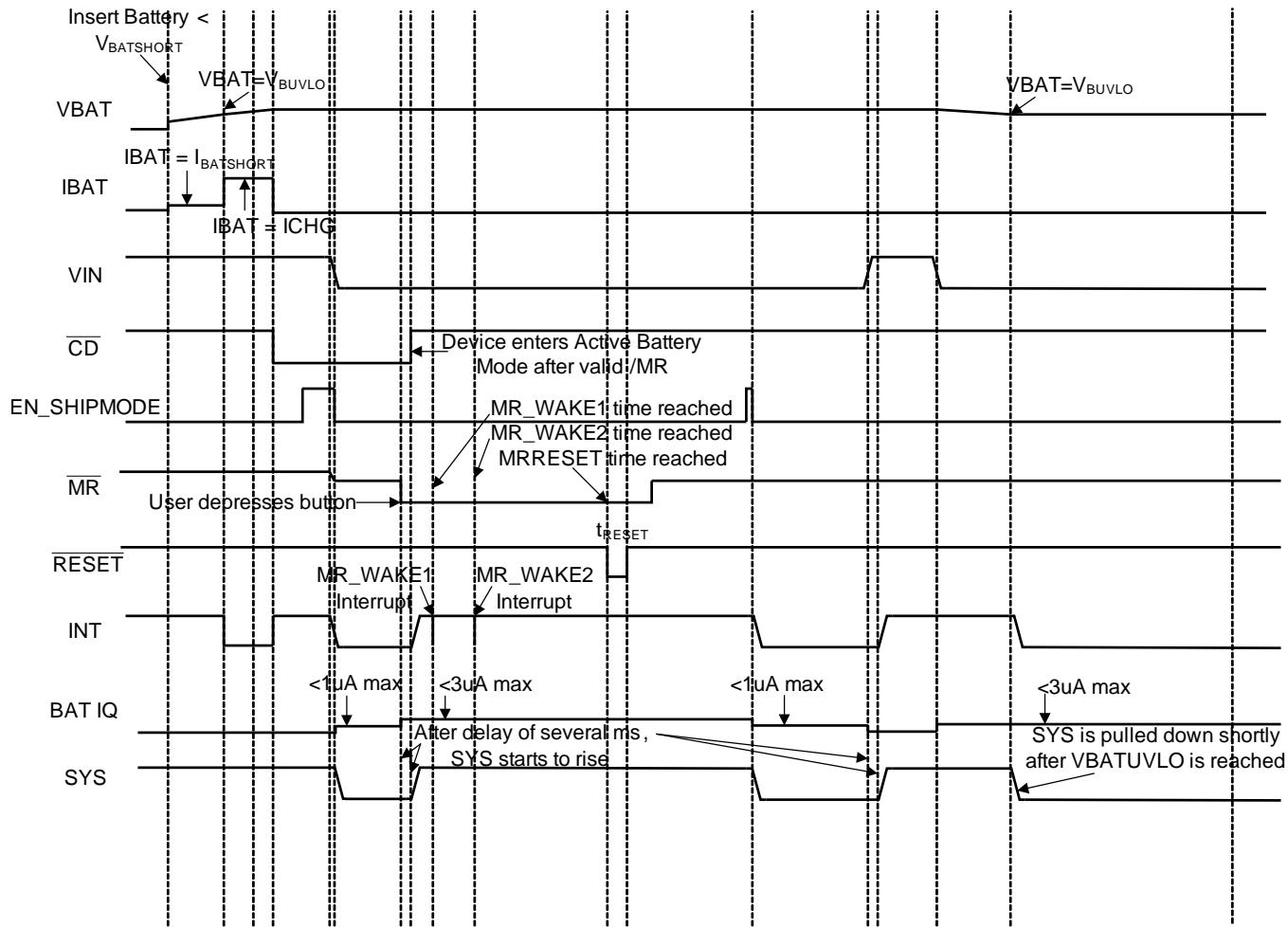
**図 2. Battery Operation and Sleep Mode**
