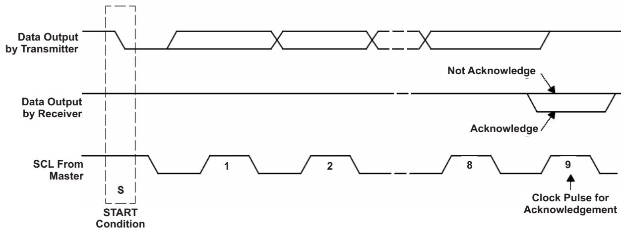
**图 21. Acknowledge on the I<sup>2</sup>C Bus**
