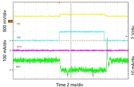
**図 42. Charger On/Off Using  $\overline{CD}$**
