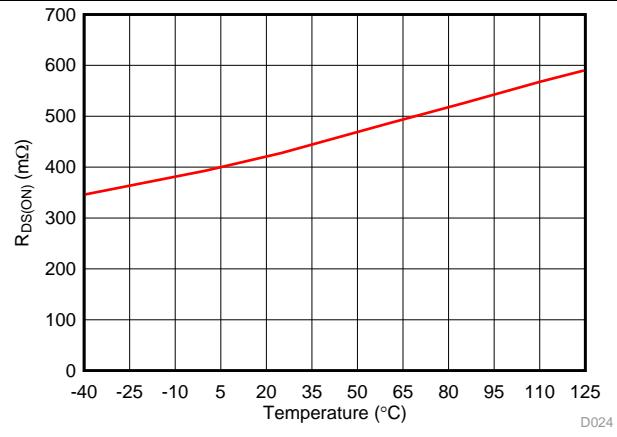
**図 6. Blocking FET  $R_{DS(ON)}$  vs Temperature**
