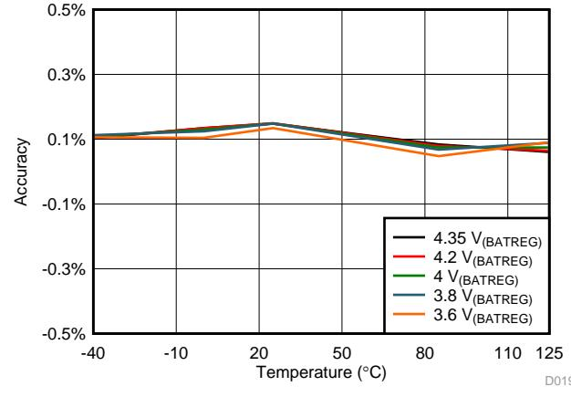
**図 8.  $V_{BATREG}$  Accuracy vs Temperature**
