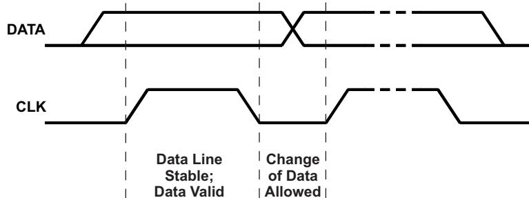
図 20. Bit Transfer on the Serial Interface
