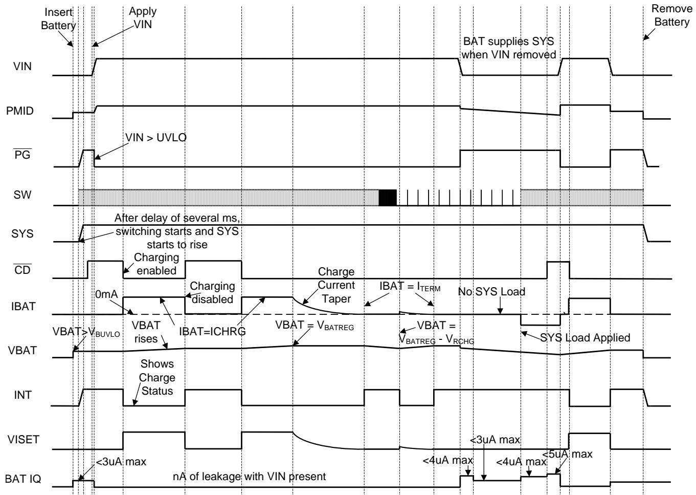
Conditions: PGB\_MRS = 0, TE = 1, SW\_LDO = 1, VINDPM\_ON = 0, PG and INT pulled up to SYS, EN\_INT = 1
