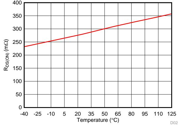
**図 7. Battery Discharge FET  $R_{DS(ON)}$  vs Temperature**
