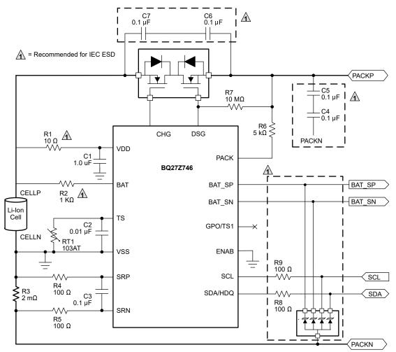
図 8-1. BQ27Z746 1-Series Cell Low Side Current Sensing Typical Implementation
