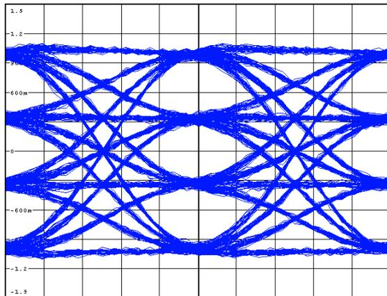
1 Mbps 4-GFSK, 400-kHz Deviation, 500-kHz Loop Bandwidth
