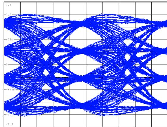
1 Mbps 4-GFSK, 400-kHz Deviation, 300-kHz Loop Bandwidth
