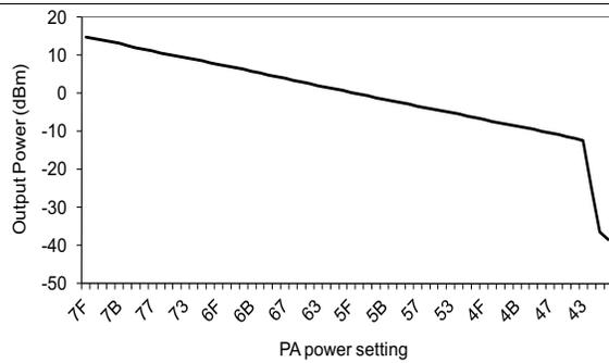
**Figure 4-9. Output Power at 868 MHz PA Power Setting**
