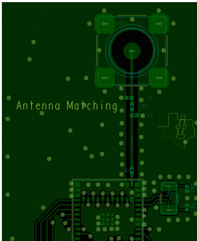
Figure 10-5. Module Layout Guidelines with External Antenna
