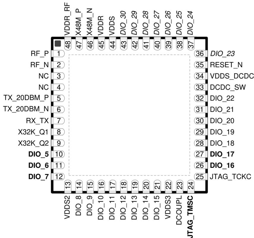
❑ 6-1. RGZ (7-mm x 7-mm) Pinout, 0.5-mm Pitch (Top View)
