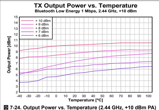
Fig 7-24. Output Power vs. Temperature (2.44 GHz, +10 dBm PA)
