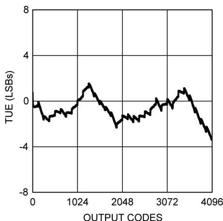
図 7-3. Total Unadjusted Error vs Output Code
