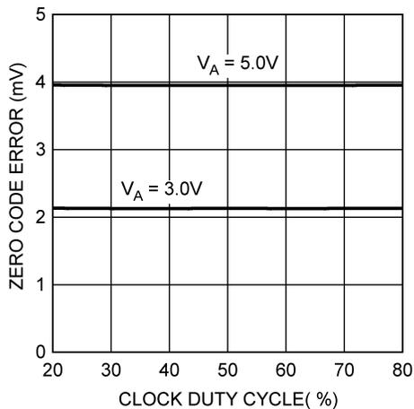
5-20. Zero Code Error vs Clock Duty Cycle
