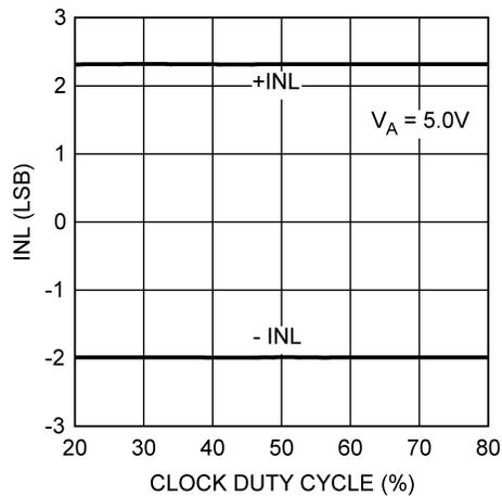
图 5-16. 5V INL vs Clock Duty Cycle
