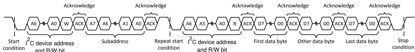
Figure 7-8. Multiple-Byte Read Transfer
