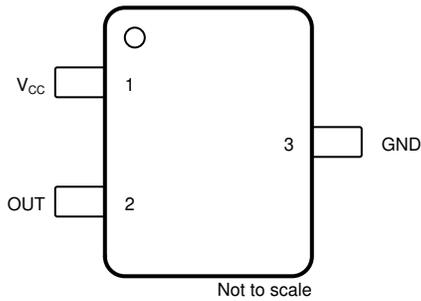
✎ 5-1. DBZ Package 3-Pin SOT-23 Top View
