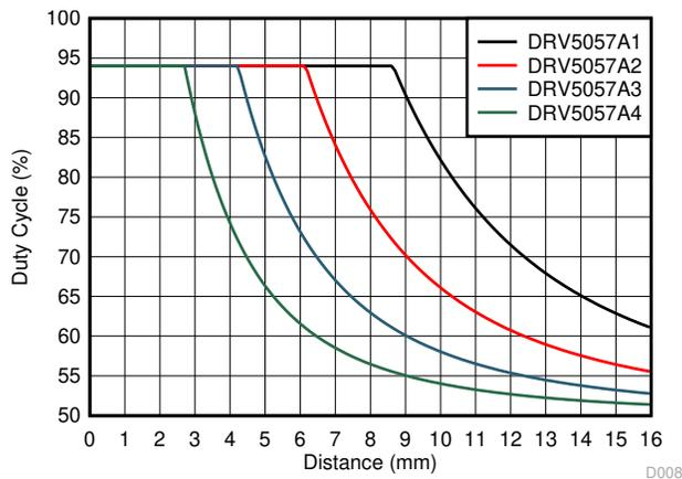
**Figure 8-7. %D vs South Pole Distance (All Gains)**
