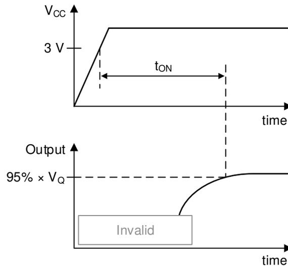
**Figure 7-4.  $t_{ON}$  Definition**
