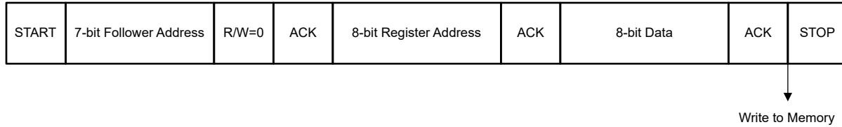
図 8-20. I 2 C Write Sequence
