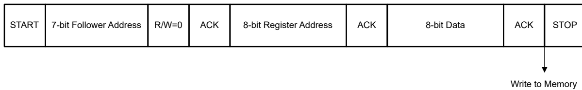
図 7-21. I 2 C Write Sequence
