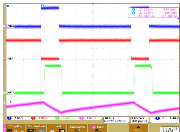
9-9. Driver delay compensation (1.8 μs)
