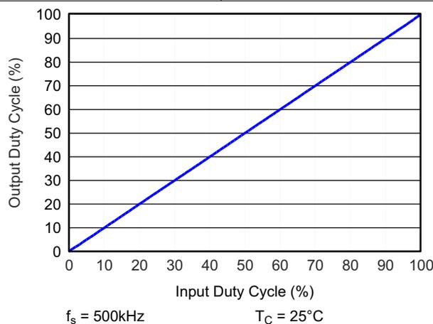
图 5-5. Output Duty Cycle vs Input Duty Cycle
