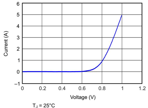
图 5-4. Drain To Source Diode Forward On Characteristics
