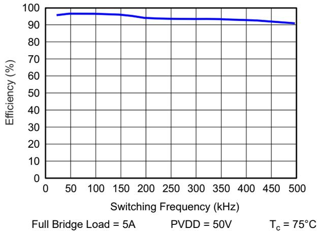
图 5-1. Efficiency vs Switching Frequency (DRV8432)
