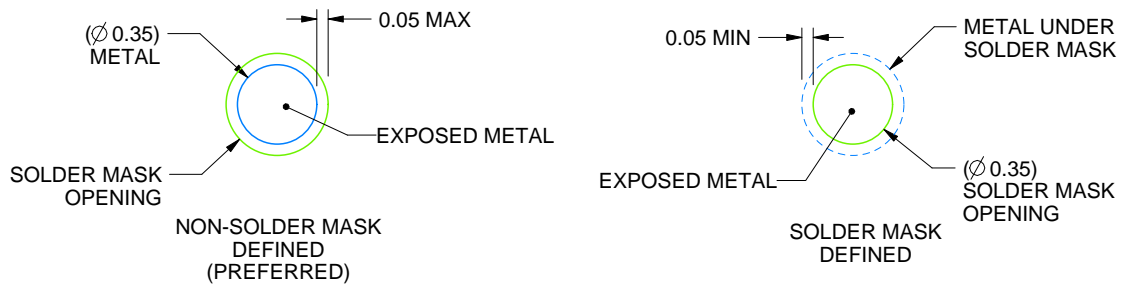
SOLDER MASK DETAILS NOT TO SCALE
