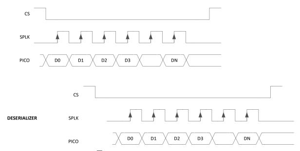
図 7-2. Forward Channel SPI Write
