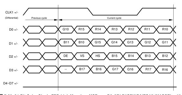
図 7-20. 24-Bit Color Single FPD-Link Mapping: MSBs on D3, "OLDI/SPWG/VESA" (MAPSEL = H)
