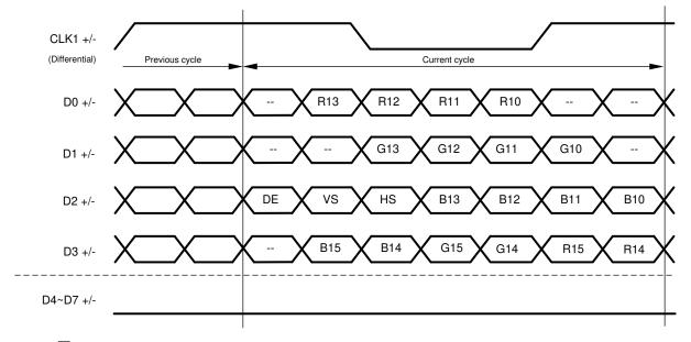
図 7-24. 18-Bit Color Single FPD-Link Mapping, "4 Lane 18 Bit Mode" (MAPSEL = H)
