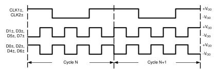
図 6-1. Checkerboard Data Pattern
