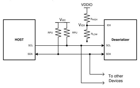
図 7-28. Serial Control Bus Connection
