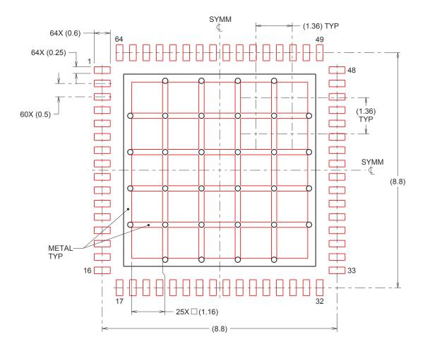
図 10-1. 64-Pin WQFN Stencil Example of Via and Opening Placement (Dimensions in mm)
