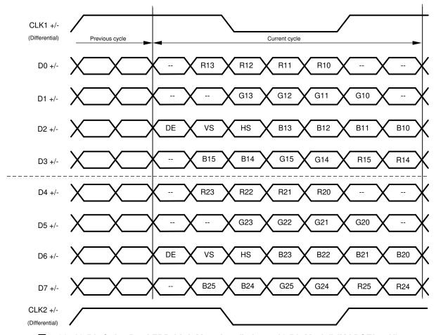
図 7-22. 18-Bit Color Dual FPD-Link Mapping, "4 Lane 18 Bit Mode" (MAPSEL = H)
