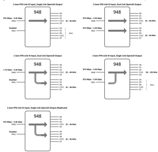
**図** 7-15. Data-Path Configurations
