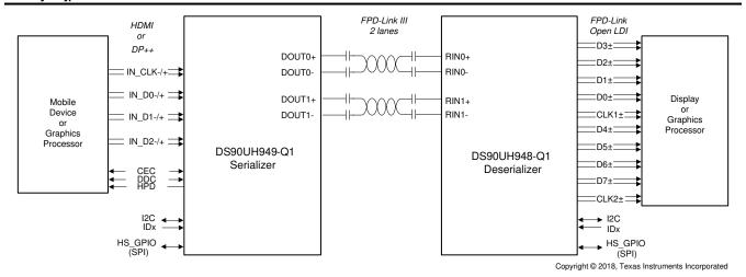
図 8-3. Typical Display System Diagram
