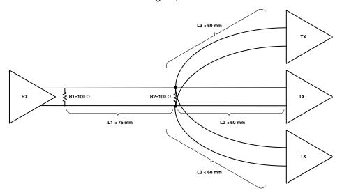
図 7-12. FPD-Link Fan-Out Electrical Requirements
