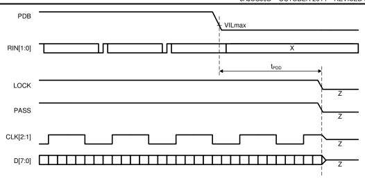
図 6-5. FPD-Link and LVCMOS Power Down Delay
