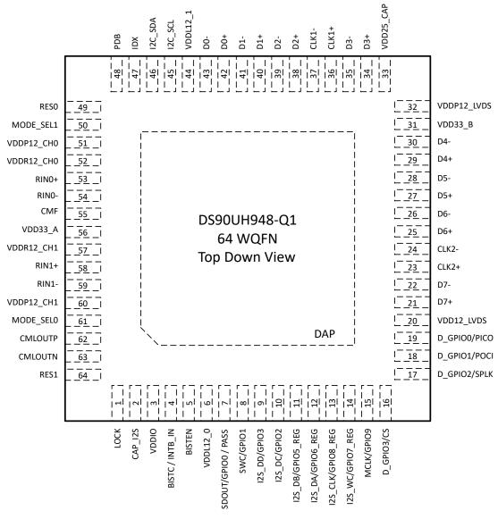
図 5-1. NKD Package 64-Pin WQFN Top View
