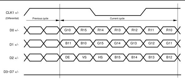
図 7-25. 18-Bit Color Single FPD-Link Mapping, Standard 18 Bit (MAPSEL = L)
