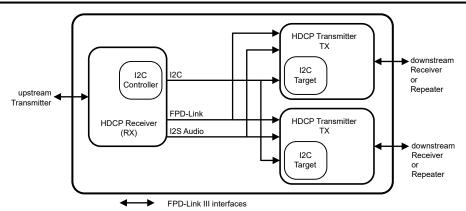
図 7-10. HDCP 1:2 Repeater Configuration
