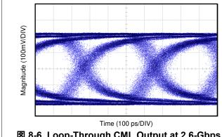
図 8-6. Loop-Through CML Output at 2.6-Gbps Serial Line Rate
