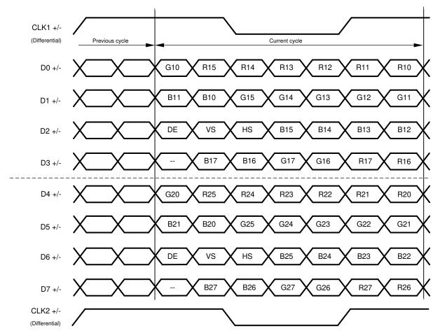
図 7-18. 24-Bit Color Dual FPD-Link Mapping: MSBs on D3/D7,"OLDI/SPWG/VESA" (MAPSEL = H)
