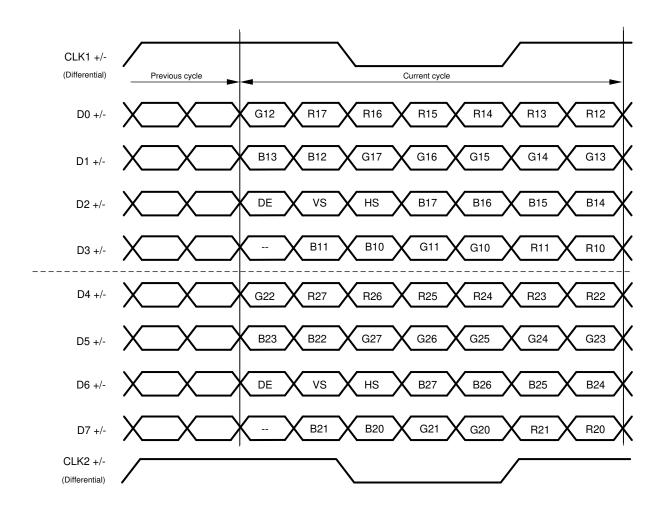
図 7-19. 24-Bit Color Dual FPD-Link Mapping: LSBs on D3/D7, "JEIDA" (MAPSEL = L)
