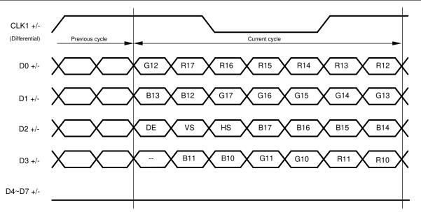
図 7-21. 24-Bit Color Single FPD-Link Mapping: LSBs on D3, "JEIDA" (MAPSEL = L)
