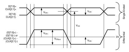
図 6-9. FPD-Link Single-Ended and Differential Waveforms
