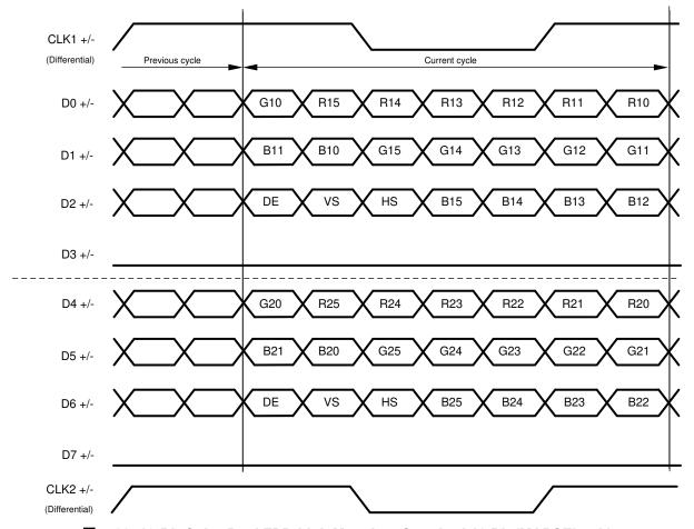
図 7-23. 18-Bit Color Dual FPD-Link Mapping, Standard 18 Bit (MAPSEL = L)
