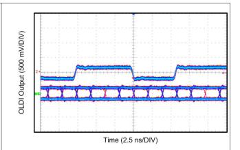
図 8-7. OpenLDI Clock and Data Output at 74.25-MHz Pixel Clock
