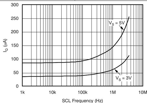
**Figure 12. Shutdown  $I_Q$  vs  $I^2\text{C}$  Clock Frequency**
