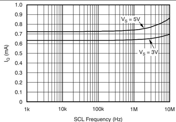
**Figure 11. Active  $I_Q$  vs  $I^2\text{C}$  Clock Frequency**
